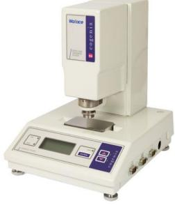
The Wallace H14 is a digital, bench-mounted hardness tester designed for measuring in IRHD the hardness of standard rubber samples.
