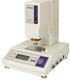
The Wallace range of H17 digital, bench-mounted hardness testers is designed for measuring in Shore scale the hardness of various materials. Four models are offered – the H17A for testing standard rubber, H17O for soft rubber and medium density textiles, H17D for hard rubbers and plastics and H17M for thin/small rubber samples.
